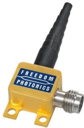
Figure 11. (Left) Photograph of a packaged 22 GHz photodiode module with a pigtailed optical fiber input and V-type connector. (Right) RF power vs. frequency for a fully packaged device, with a responsivity of 0.45 A/W. The 3-dB bandwidth of this device ranges between 15 and 25 GHz, depending on incident optical power. Responses are shown for photocurrents ranging from 0.5 mA to 10 mA. Circles show the data; lines overlaid are polynomial fits.
